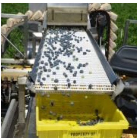
Fig. 4. Fruit bruising occurs when the fruit falls from a distance to a hard surface.
