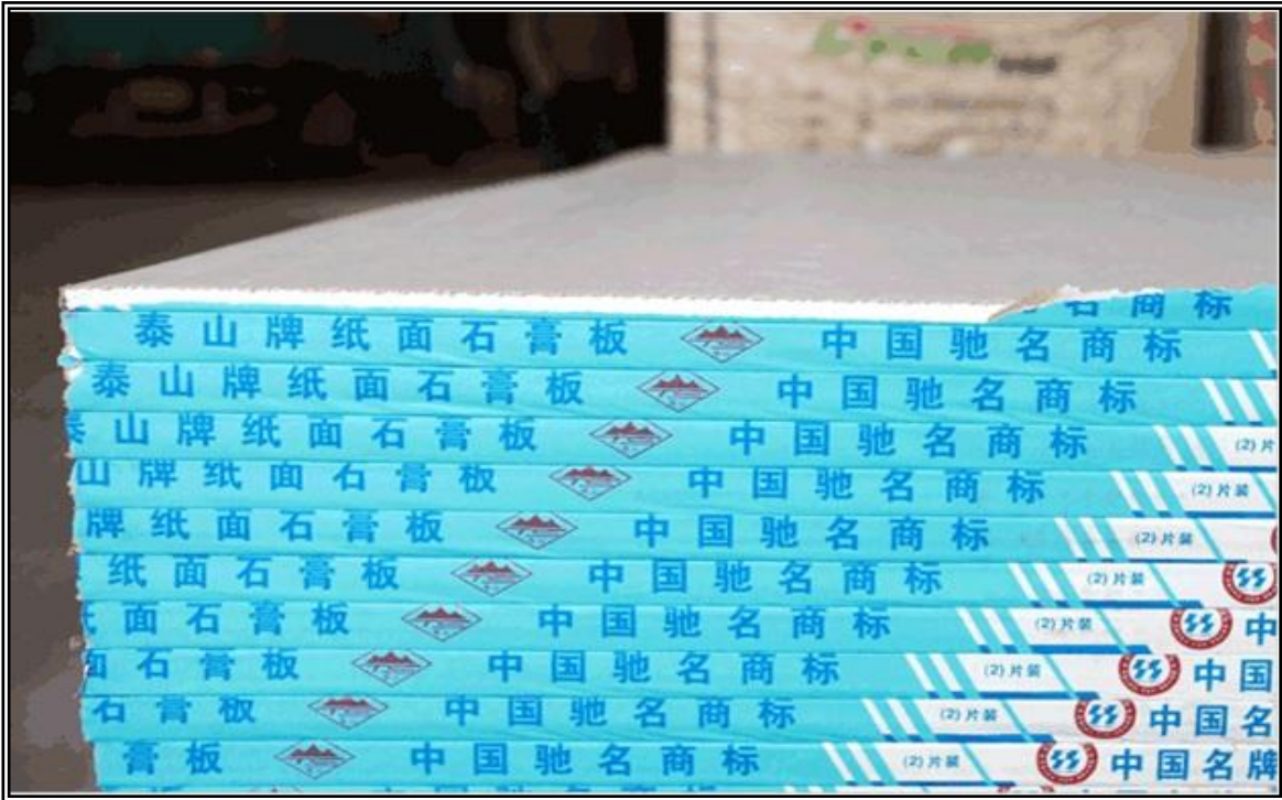
Photo 1: Most corrosive drywall was imported from China between 2005 and 2007.
