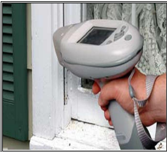
Photo 3: On-site XRF analysis can be helpful for locating corrosive drywall panels, but several factors must be considered in data interpretation.
