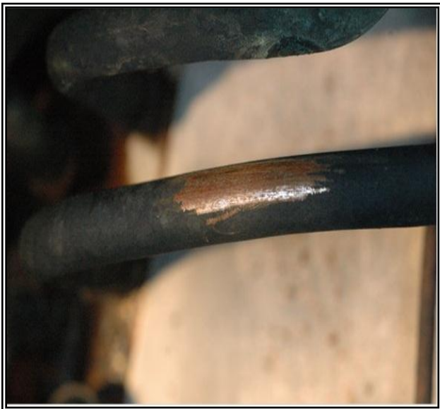
Photo 2: Blackening of copper surfaces indicates sulfur corrosion.
