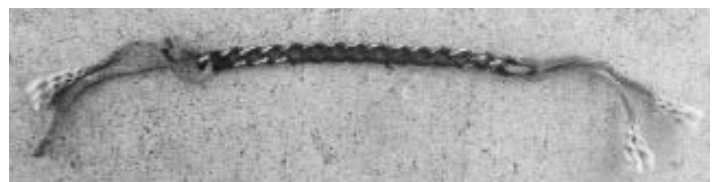
Unacceptable curb chain strap
