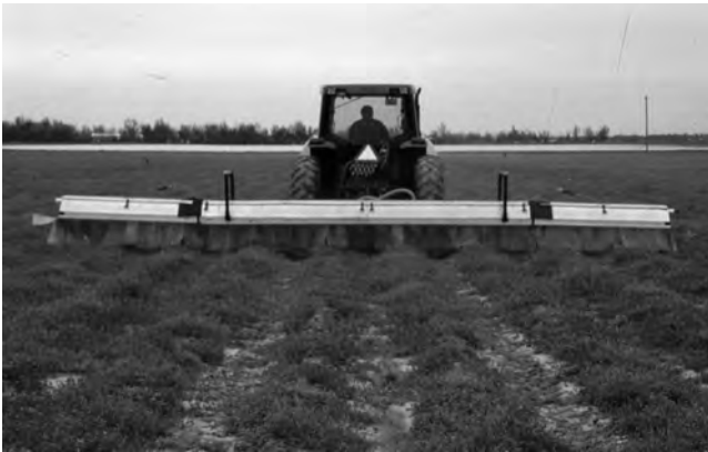
Figure 6. Broadcast shielded sprayer operating in “burn-down”
