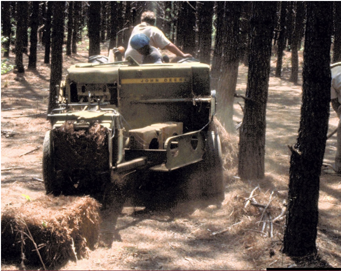
Figure 2. Mechanical baler along windrow. Photo by David J. Moorhead, University of Georgia, Bugwood.org.
