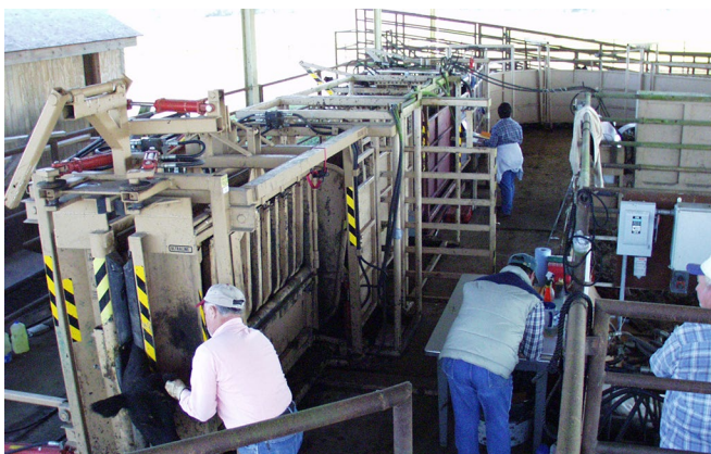
Figure 6. Slider (alley divider) extended outward between palpation cage and scale compartment.
