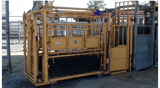
Figure 16. Scales mounted under squeeze chute.
