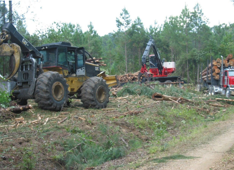
Figure 12. Typical logging equipment: grapple skidder, loader, and trees loaded on a truck awaiting transport. Photo by James Floyd
