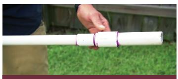
**Step 4:** Glue a 6-inch section of 1½-inch PVC pipe to each end of a 1-inch-wide, 20-foot-long PVC pipe using the PVC reducing couplings.
