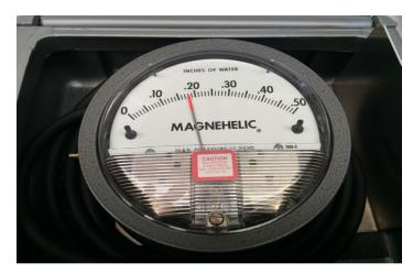
Figure 1. Hand-held Magnehelic static pressure gauge.
