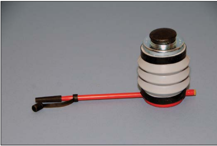
Figure 10. This bulb duster is used to blow dust into colonies of bees in buildings or protected cavities. It may be difficult to find locally but can be readily ordered from Internet sources. (Photo by Blake Layton)
