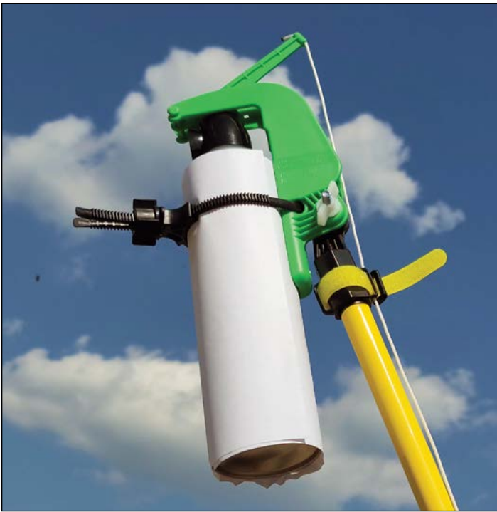
Figure 12. This Gotcha Sprayer is connected to a telescoping pole that allows application of aerosol insecticides to honey bees nesting overhead without climbing a ladder. The applicator pulls the twine, and the hinged, green lever depresses the top of the spray canister (wrapped in white paper to conceal brand name) to release the insecticide. (Photo by J. W. Harris)
