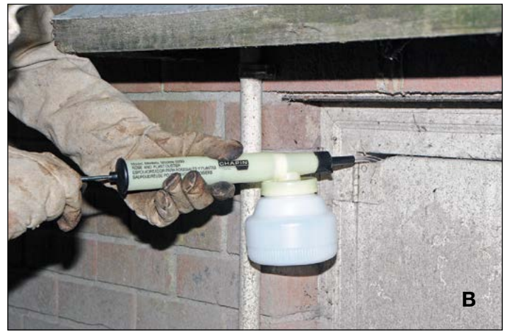
Figure 9. This garden duster is used to blow dust into colonies of honey bees in structures: (A) fitted with a small hose; and (B) inserted into a void to direct dust onto a bee nest. (Photos by Blake Layton)
