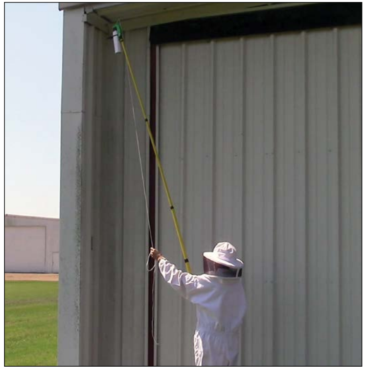
Figure 12. This Gotcha Sprayer is connected to a telescoping pole that allows application of aerosol insecticides to honey bees nesting overhead without climbing a ladder. The applicator pulls the twine, and the hinged, green lever depresses the top of the spray canister (wrapped in white paper to conceal brand name) to release the insecticide. (Photo by J. W. Harris)
