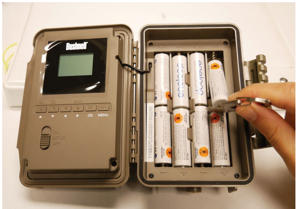
Figure 9. Replacing batteries using a multi-tool. (Photos by Eden Blackwell/University of Alabama)
