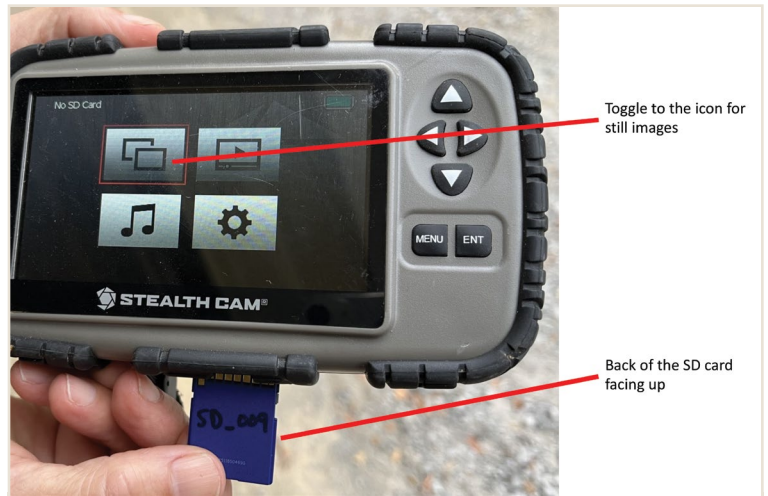
Figure 6. Insert SD cards into the SD reader with the back of the card facing up. (Photo by Ann Smithson/ Mississippi State University)
