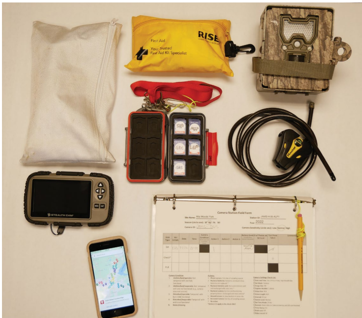
Figure 16. Basic components of volunteer camera kits. (Photo by Eden Blackwell/University of Alabama)
