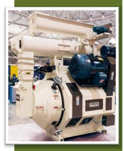
Large electric motors are used to power pellet mills, which compact wood particles and extrude them as pellets through small openings in steel dies.
