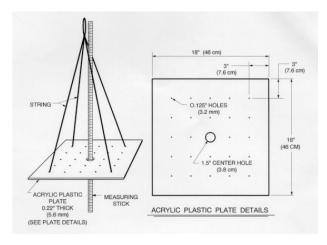
Figure 2. Falling plate meter schematic (Rayburn and Lozier, 2003.)
