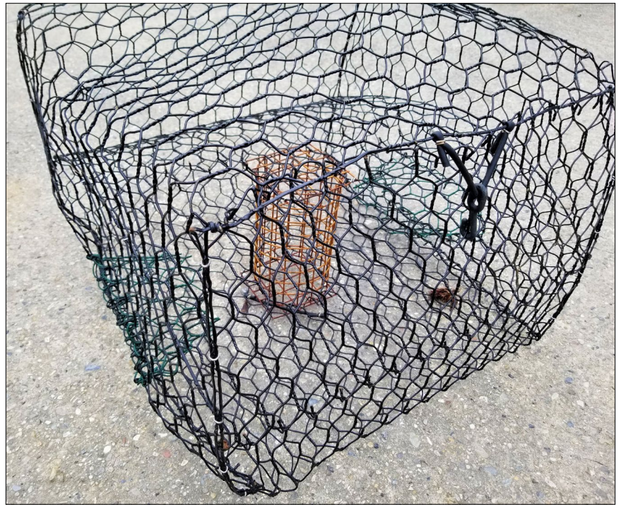
A standard wire crab trap used to fish for blue crab. The orange wire pocket holds bait (menhaden or catfish are common choices) and sits on the sea floor. The green wire entrances lure in unsuspecting crabs. To empty the trap, the user unhooks the top from the side and shakes the contents out. Photo credit: Sarah Cunningham, Coastal Research & Extension Center.
